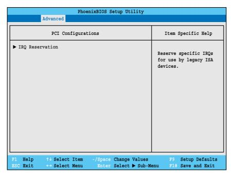
Figure 8. PCI Configurations Submenu
